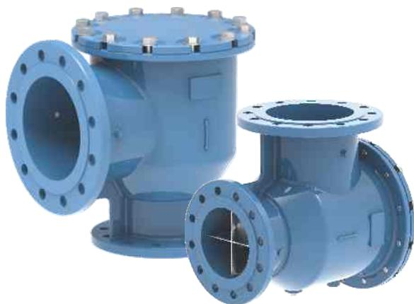
The **NORTHAM** NG-T series Triple Duty Valves save space and reduce purchase and installation costs by combining all the functions normally required on the discharge side of most HVAC systems into one convenient design. It features a calibrated balance valve, non-slam check valve, and positive shut-off valve, all combined into one.
